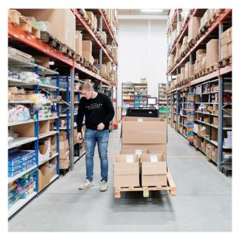
When a round of picking starts, the employee receives information about the sizes of packaging to take on the picking cart and the specified position of the boxes on the cart. Labels for each order are printed automatically and then attached to the packages. As the goods are picked, they are placed directly into the shipping packaging, which is on the picking cart.
