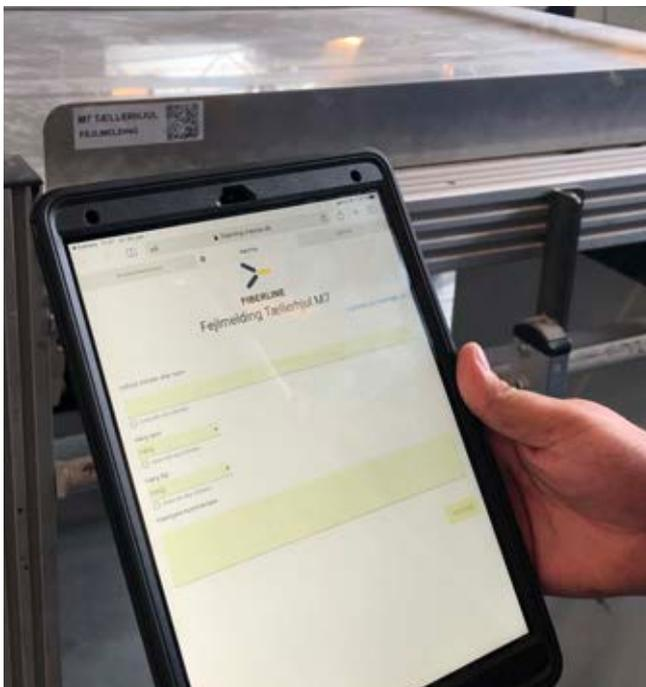
When an operator submits a job request from the production, he uses the product line's tablet to scan the QR code on the machine and fill out the predefined fields. This ensures that all job requests are documented and executed. This solution makes sure that no tasks are forgotten or left behind.
